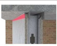
CEMCO HOTROD XL fire rated drywall accessory
