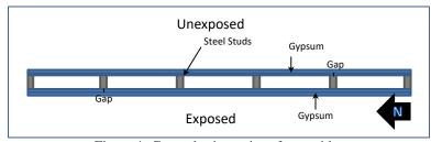
Figure 1. General schematics of assembly.
